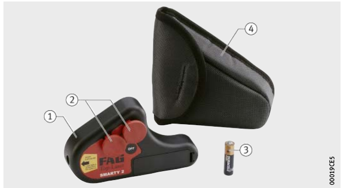
Figure 2 Scope of delivery FAG Top-Laser SMARTY2
