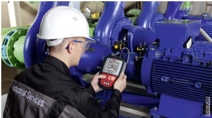
Figure 6 Shaft alignment device FAG Top-Laser EQUILIGN
